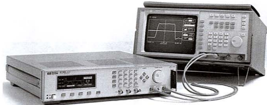
Typical HP 8110A pulse generator stimulus-response set up with the HP 54503A oscilloscope for testing analog and digital circuits up to 150 MHz.
