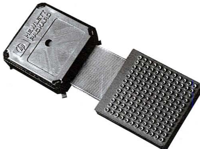
HP's low-profile adapter for probing soldered-on, surface-mounted microprocessors.
