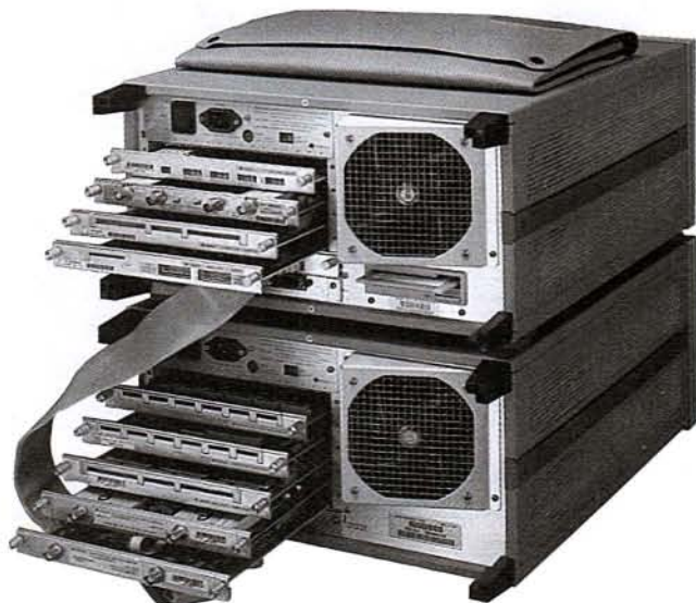
The HP 16500A supports nine different measurement modules.
