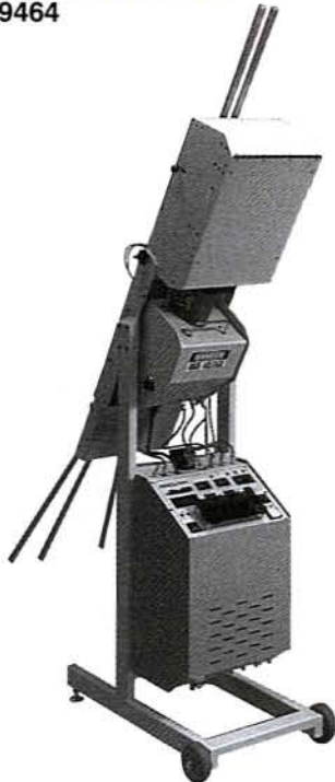
HP 9464 integrated with a tube-to-tube DIP handler
