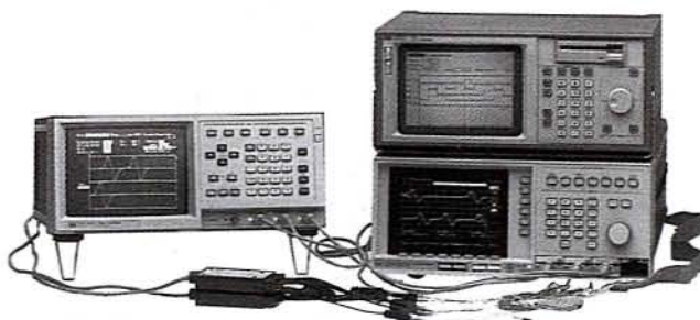
HP 8175A starts HP 1650A logic analyzer and HP 54110D oscilloscope signal capture.
